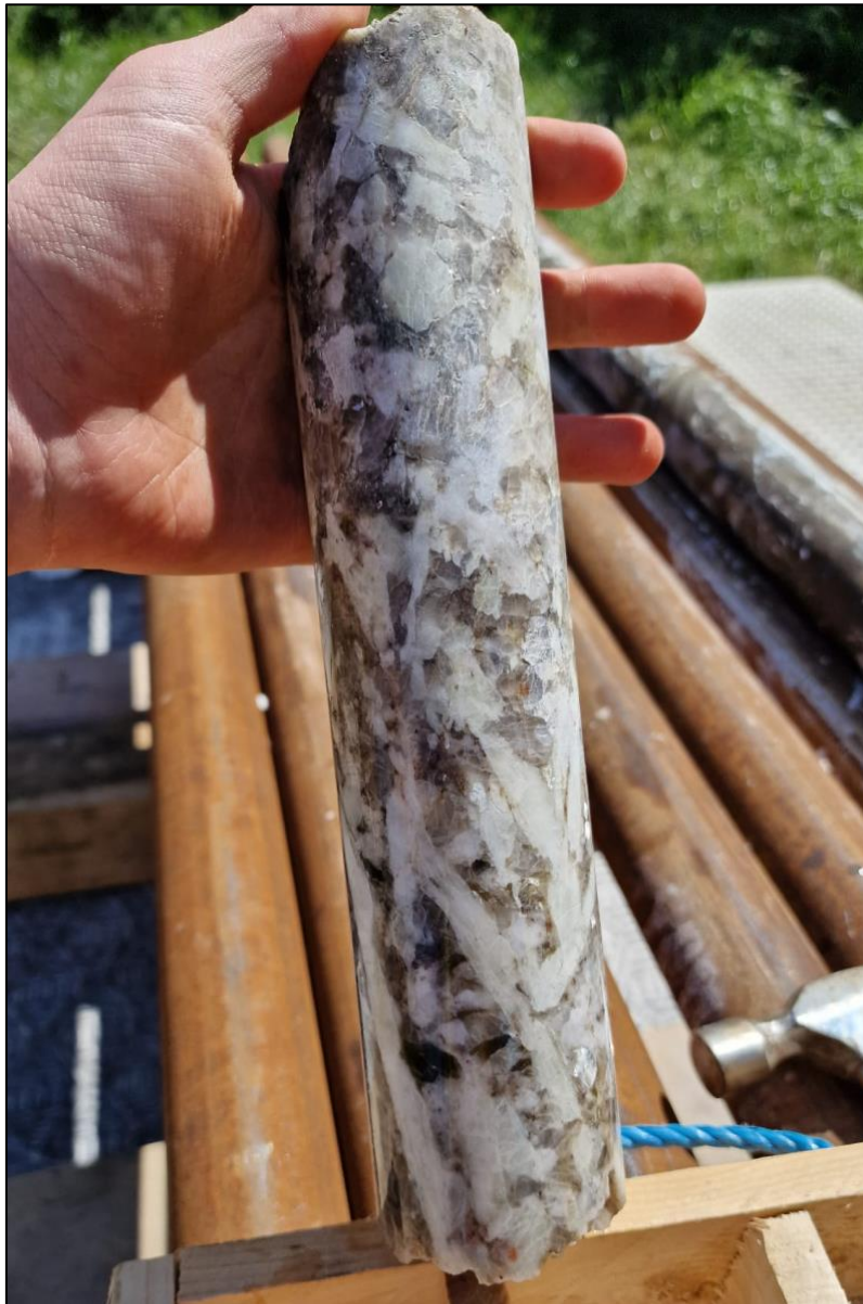
Image 2: Spodumene pegmatite in drill core DDH 23-1597-02
