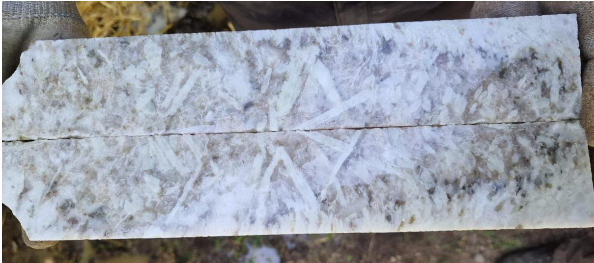
Image 1: Spodumene pegmatite in drill core DDH 23-1597-01
