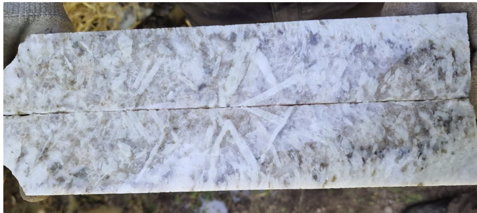
Spodumene pegmatite in drill core DDH 23-1597-01 (PEG-01 [part of]; 34.59-34.94. Sample AES65107 reporting intercept apparent thickness of 0.36m \ True thickness 0.05m @ 2.95% Li 2 O)
