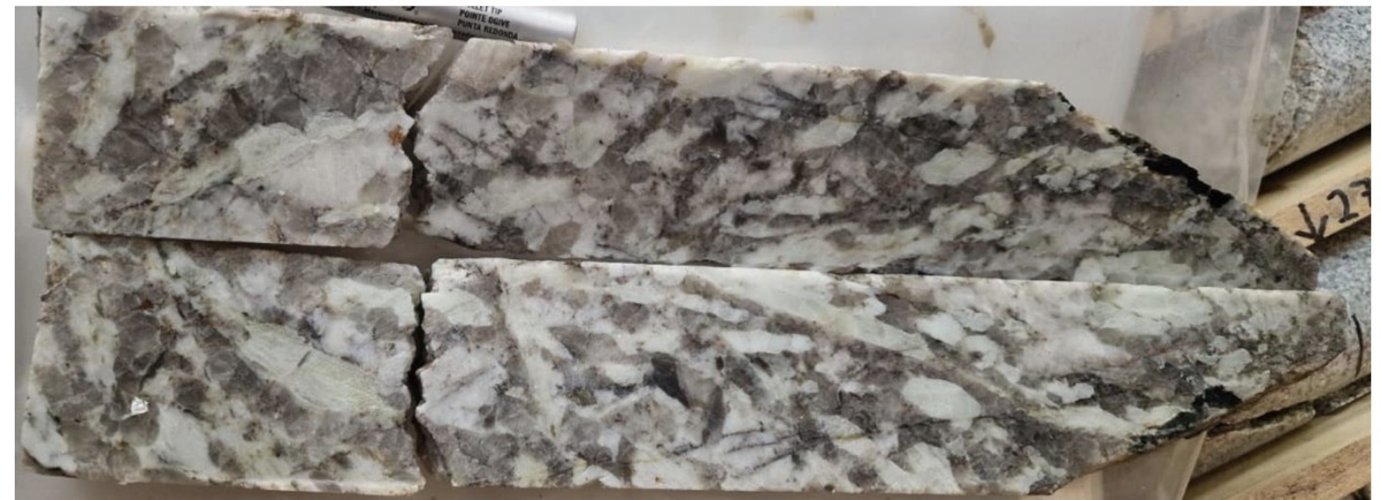
Spodumene pegmatite in drill core DDH 23-1597-02 (PEG-04; 31.46-31.85. Sample AES65136 reporting 0.39m @ 1.59% Li 2 O)
